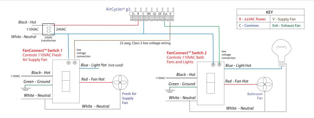
By using the AirCycler® g2 to control both an exhaust fan, such as the bathroom fan, and a fresh air supply fan, the fresh air supply can be programmed to run a set number of minutes every hour to provide for required mechanical ventilation. If desired, the bath fan can be activated at the same time to provide a "balanced" ventilation strategy.
