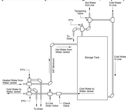
water jacket, the tank must be at least two feet higher than the water jacket.) Locate the storage tank within eight horizontal feet of the water jacket. For optimum performance, place the tank as high above the stove as possible.
