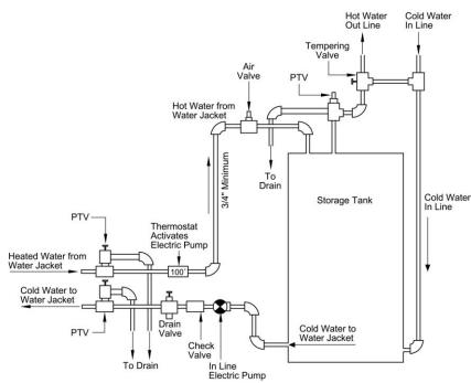
Caution: In the event of a power failure, water may stop moving and become highly pressurized in the water jacket and piping. An additional pressure temperature relief valve (PTV) must be located in the hot water line within two feet of the water jacket. The PTV must be installed according to local building and safety codes, and must be piped to a drain.
